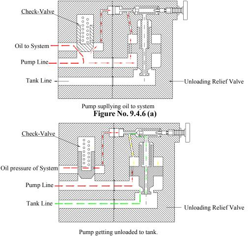
Unloading valve is always used with a check valve a shown in figure.
