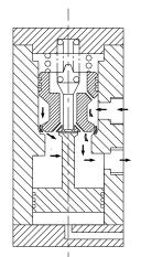
Pilot operated check valve full flow in reverse direction
