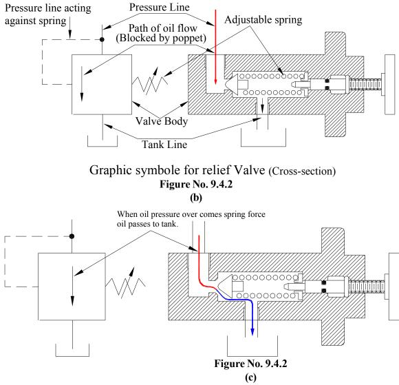
As oil pressure overcomes spring force, oil passes by to tank. (Second figure is only explanatory drawing. In actual as oil port of pressurized oil is always block in normally operating condition. Hence in hydraulic symbol also the path of oil will always be shown as off-centered and blocked).
