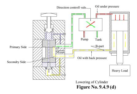
While lowering load, oil coming out from B-port gets resistance from spring, and only developing pressure sufficient to lift the spring oil gets exhausted to tank via primary port and direction control
