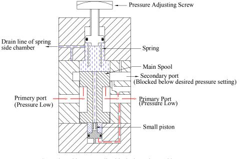
Secondary side pressure line blocked as primary side pressure is below the required
