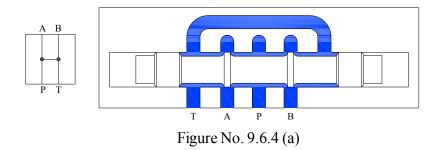
**2.** Close-Center Type: - In this type all the ports are blocked. Pump port is blocked hence pressure develops. Oil passes over relief valve or used for operating other valves.
