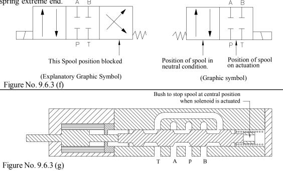
**5.** Two Position Detente: - Similar to the three position spring centered valve this valve also have two actuator but without spring. And it has arrangement to keep the spool to its extreme end even when actuator released. Hence when actuator is shifts the spool it remains in same position, do not return to neutral position even when actuation released. And will pass on to other extreme position when other actuator actuated.
