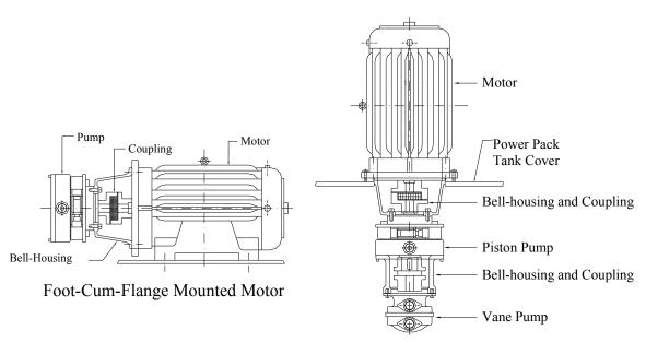
Vertical Flange Mounted Motor Figure No. 9.2
