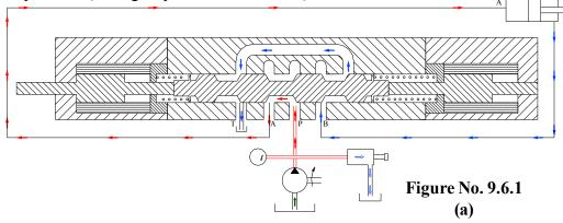
Spool shifted to other extreme end, and at this position it connects pump to cover end of cylinder, and tank to front end of cylinder. Cylinder takes its forward stroke and oil from front-end returns to tank. Working pressure will be as per pressing load on cylinder.
