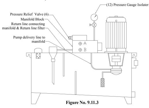
A single manifold block or sub-plate is block which has connection port for connecting pump, exhaust port, and two oil port for cylinder, and on its various ground surface provision to mount the valves.
