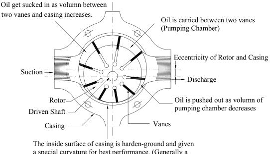
a special curvature for best performance. (Generally a harden and ground ring called Cam-ring is fitted inside for convenience in maintenace and replacement of worn out ports) **Figure No. 9.3.3**
