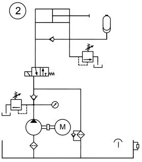
Piston rod is connected to fluid gate of Dam. When ever system switched off purposely or by power failure, piston-rod retracts back and opens the fluid gate **3)** Energy and safety:- An accumulator which is kept always in fully charged condition, gives instant power for safety operation, such as breaking, closing or opening of door etc. (Pump take few seconds for developing rated pressure, while accumulator keeps it in ready stock for instant supply.)
