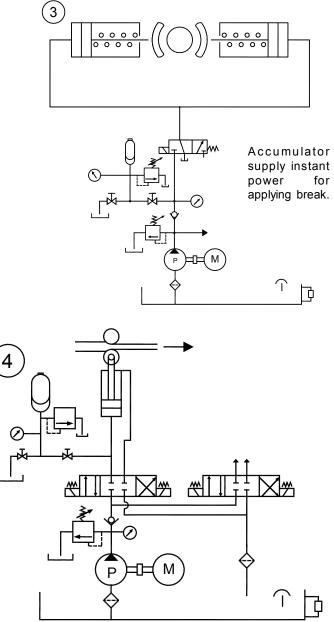
Accumulator supply costant pressure on rolls of rolling machine.
