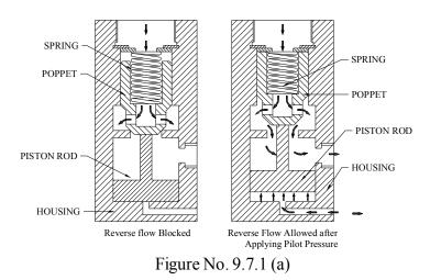
As pilot operated check valve is used to hold the high-pressure oil locked in cylinder. Suddenly releasing the oil pressure from cylinder will produce a shock and vibration, which are damaging the system.
