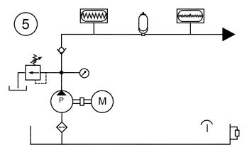
Accumulator dampens the pulse generatd by pump.
