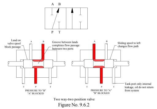
In case of four-way valves, oil also returns to direction control valve and flows through the tank port to tank. In one position of spool, oil flows from pump to port-A, and port-B to tank, and in other position oil flows from pump to port-B and port-A to tank. The valve discussed earlier (figure 30.2) is a four-way valve.
