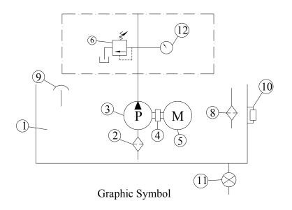
Pressure Gauge (12) Pressure Gauge Isolater (12) (5) Moter Direction control valve (7) Pressure relief valve (6) A & B is Oil Port for Cylinder or Moter (13) đ Return line filter (8)  $\oplus A$ Filler (9)  $\oplus B$ (4) Coupling breather  $\boxtimes$ (10) Oil level J indicator Tank (1)-(3) Pump (2) Suction filter (11) Drainer Figure No. 9.11.4 В A Р Т (6) (9 103 (1)2 4 (8)(11)Figure No. 9.11.5
