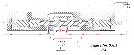
Spool of direction control valve shifted to one extreme end, because of which a path for oil open between pump to return port-B, of cylinder, and tank to forward port-A, of cylinder. Cylinder starts retracting and oil from cover end of cylinder passes on to tank.
