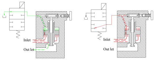
(1) Vent port connected to tank through solenoid valve. Because of which pilot operated relief valve unloading full discharge of pump to tank, and there is no pressure in hydralulic system. (2) As soon as solenoid valve gets enegied, it block the vent port. And pilot operated relief valve stop by-passing to tank, and pressure get developed in system.
