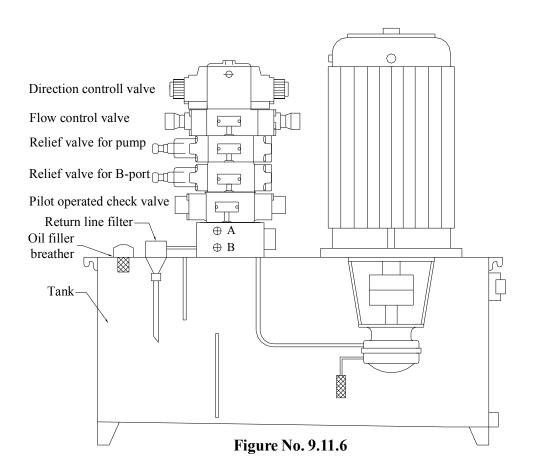
In following example we have added many modular valves such as, flow control valve, pilot operated check valve, pressure relief valve for both A & B port. The valve used in said power pack unit add following feature in power pack.
