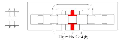
**3. Tandem Type: -** In this type both the oil port for cylinders are blocked and pump port is connected to tank. Hence in neutral position cylinder remains locked while pump is unloaded to tank at low pressure. These types of valves could be connected in series.
