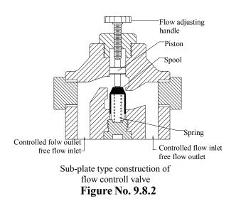
Manufacturing a hydraulic system becomes simplest using such types of valves. But this type of construction has limited flow capacity. As largest type of valve is only as per CETOP-5, hence their maximum flow capacity is only 100 LPM. And best result we get only below 40 LPM and 200 bar working pressure.
