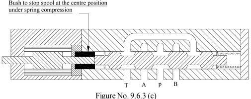
By actuating solenoid spool will be pushed against spring-to-spring end, and on releasing it will return to center. As on actuator end there is a stopper hence it cannot over travel to actuator end by spring force.
