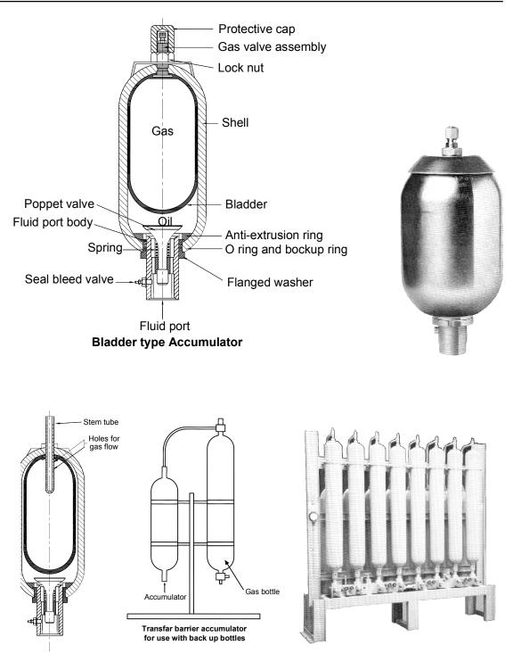
Transfer barriers accumulators are those in which compressed gas section of accumulator is not locked, but connected to pressurised gas bottles or othersource of pressurised fluid. **Diaphragm type Accumulator:** - Diaphragm type accumulators are similar to bladder type accumulator with two following differences:
