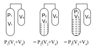
Accumaltor capacity =  $V_f = V_2 - V_3$
