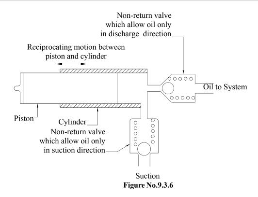
In outward stroke of piston, cylinder sucks fluid, and in inward motion of piston, cylinder delivers fluid. Similar numbers of small pumping units are used in one piston pump. The mechanism to reciprocate piston differs in different type of pump.
