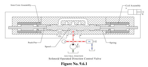
Direction control valves at central position and in this configuration or type the spool is blocking both the port of cylinder, pump as well as tank and all the flow of oil supplied by pump is returning to tank after passing over relief valves. Pumps continuously run at its rated pressure (setting of pressure relief valve).
