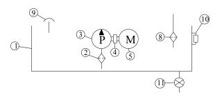
A layout should be made to decide how to fit motor, pump assembly, manifold block, return line filter, air-breather, pressure gauge etc. They should be decided, before fixing of motor-pump assembly. Once layout finalized then motor, pump assembly, and other accessories should be fixed accordingly.
