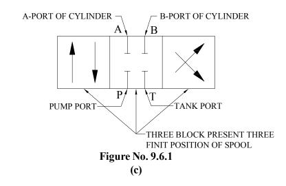
This diagram indicates at central position all ports will be blocked as we studied in circuit diagram. (30.2) On its one (left) extreme end pump will be connected to port-A and tank is connected to port-B. On its other (right) extreme end pump will be connected to port-B and tank is connected to port-A.
