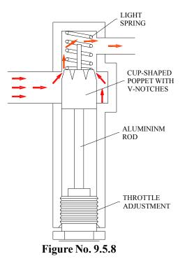
Control of flow may not be desirable in reverse flow for return stroke; hence all the flow control valves are provided a check valve for free reverse flow.
