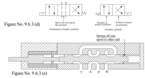
**4. Two Position Actuated to Center: -** In this configuration also spring offset spool to actuator extreme end. But when spool actuated it comes center position. It cannot pass on to spring extreme end. A B A B
