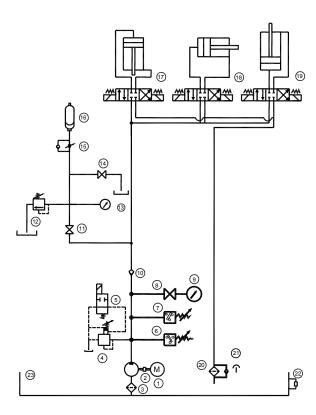
**2) Guaranteeing continuity of energy supply:-** Energy stored in an accumulator guarantees the operation of a system for specific time limit, even in case of accidental power failure.
