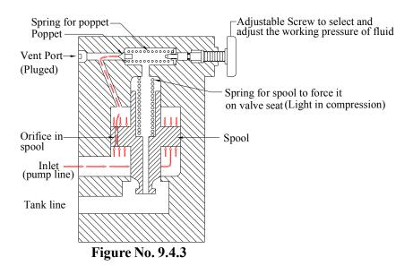
As long as poppet sits on valve seat and there is no flow of fluid across spool through orifice, pressure on both side of spool remains same. Spool remains balanced, and it also remains seated on its valve seat due to spring compression.
