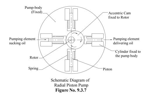
We have shown four pumping elements in our drawing, while in actual practice radial piston pump consists of 3, 5, or 7 pumping elements.
