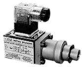
Pressure to be senced act against spring force. As pressure increases, it over-comes the spring force, and pushes the piston on one side. This cause actuation of electrical switch.
