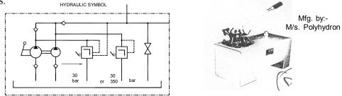
As technology progressed, hand pump also innovated and modified as per the requirement of industry. Few examples of use of hand pump are as follow:
