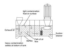
fluid level condition, sufficient fluid should be above suction point to avoid vortex or whirlpool which causes suction of air in pump. Both suction and exhaust pipe should be tapered at the end.
