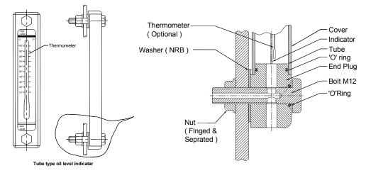
Sometimes, a thermometer is also fixed in tube type oil-level indicator to check the temperature of fluid. As in no condition temperature of fluid should exceed  $70^{\circ}$  C.
