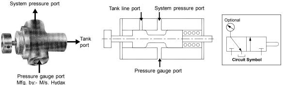
4. When a system need to read pressure at various points in multi pressure hydraulic system. Then for convenience, multi-station pressure gauge isolators are used. It replaces number of pressure gauge and single-station isolator needed to read pressure at various points.
