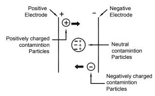
when corrugated die electric media (collectors or filter paper) are insert between electrods, the electric field between these two electrode get deformed, and die electric polarization occures at the tips of the corrugation. The electric field is strongest at the tips, and the particles are drawn and diposited on opposite electric poles and removed from oil along with die electric media (filter paper or collectore).
