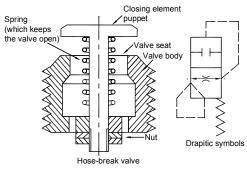
calibrated for maximum 50LPM flow rate and if flow exceeds 50LPM, then this valve will completely close the flow path of fluid and locks the actuator, cylinder or motor.
