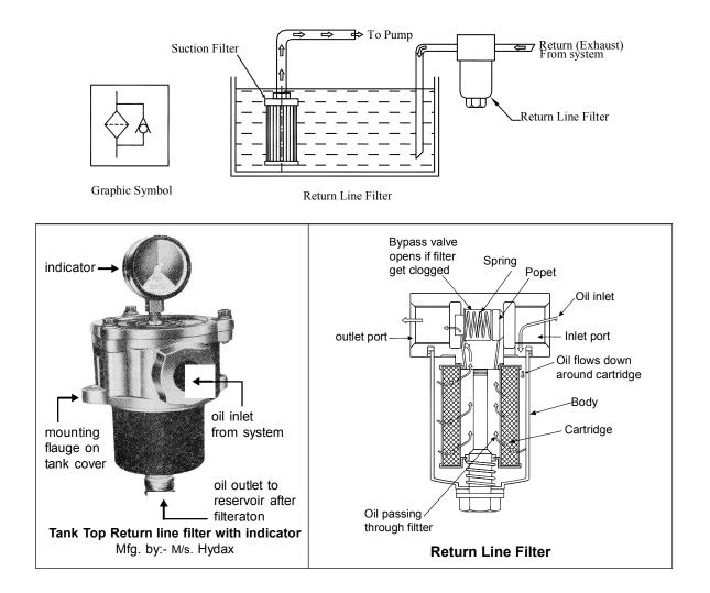
Return line filter is used at point where oil returns to tank. Depending on requirement of industry it is modified in two following ways:
