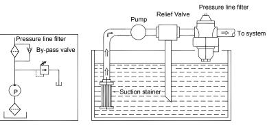
HYDRAULIC CIRCUIT DIAGRAM USING PRESSURE LINE FILTER SYSTEM USING PRESSUER LINE FILTER
