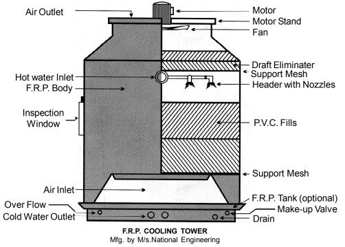
Cooling tower is also used to cool the circulating water, which is used for cooling of condenser of oil cooling chiller.
