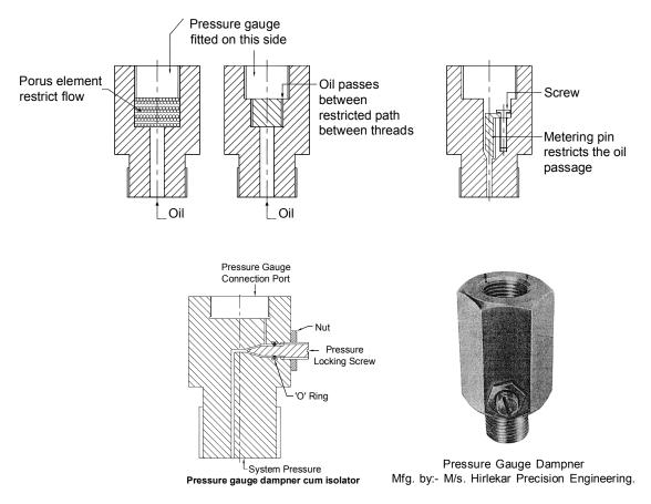
Some pulsation dampners also have features to isolate pressure gauge, similar to pressure gauge isolator. But they cannot drain pressure gauge to tank. Hence while using this unit, pressure gauge should be isolated when there is no pressure in system.
