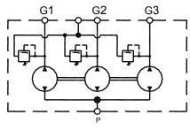
Diagram Of Three - Element Diveder With Motor
