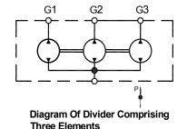
Vivolo oleodinamica of Italy manufactures a compact tendum gear pump type flow divider, which can function as a flow divider, as pump and a motor. It can synchronise number of cylinders at a time, or at act as pump, or motor for all the cylinders or individual cylinder, depending upon the configuration of flow divider and hydraulic circuit.
