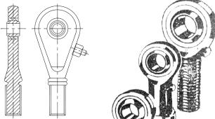
Rod end bearing with male threading
