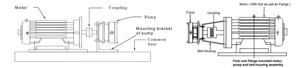
This arrangement requires large floor area, and it is too difficult to align the centre line of pump with centerline of motor. Misalignment results in damage of bearing of both motor and pump and fast wear and tear of coupling.
