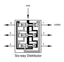
Note that no other plunger can move. i.e. only one plunger can move at a time, others remain locked, only on changing of direction does the other work. Hence this distributor are also called progressive distributor block.
