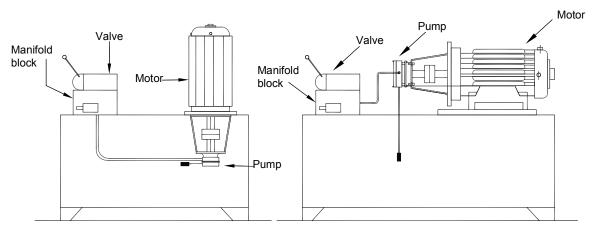
Tank top assembly type reservoir
