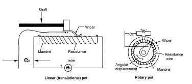
through conductor, and resistance is continuously measured by suitable electronic circuit and instrument. Any change in resistance is sensed and converted in suitable form to indicate the change in parameter which is to be measured.
