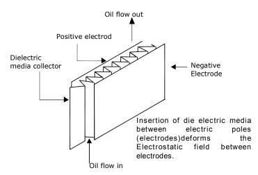
The neutral contaminations are also drawn and deposited by gradient force to the edge of the die electric media, where the intensity of the deformed electric field is the highest.
