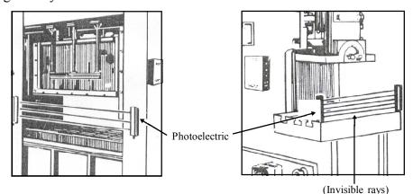
A photoelectric sensor consist of an emitter for emitting light, a receiver for receiving light. When emitted light is interrupted or reflected by the sensing object, it changes the amount of light that arrives at the receiver. The receivers detects this changes and converts it to an electrical output which is generally 10 mA current (Max). This out put current is sensed and processed by control pannel for next operation.
