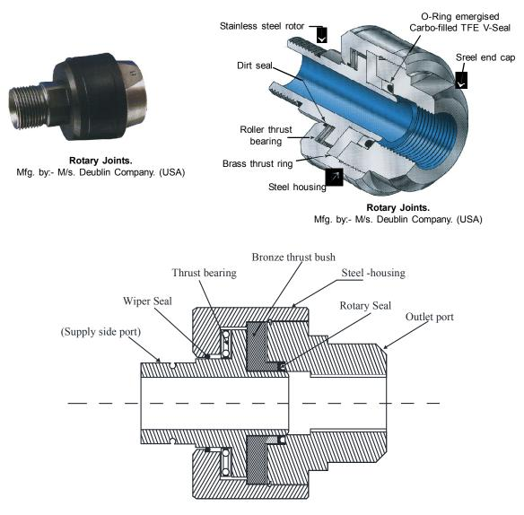
Under pressure rotary makes the joint become leak proof. Because of oil pressure outlet side port and rotor end port will try to push each other apart. It is steel honing which holds than together. To outlet port side the unit by means stationery threading. And to Rotor end side it hold the unit in place through the thrust a bearing. With stand separation face acting on both units, as well as allows relative rotational motion.
