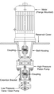
Assembly of Motor , Bell - Housing , Piston pump , Extention Bracket And Loe Pressure Pump
